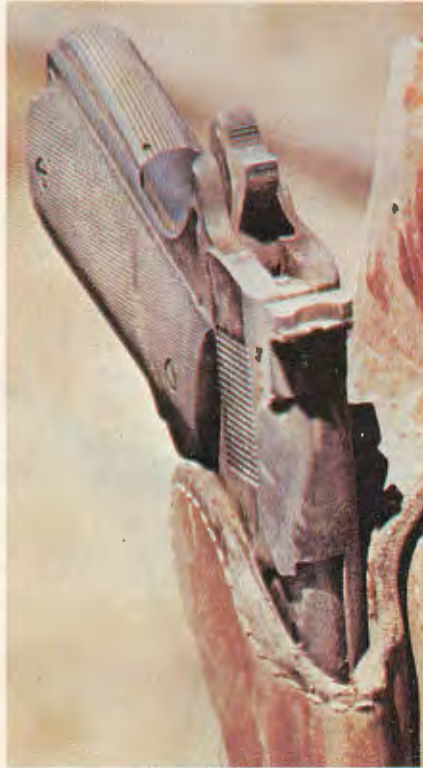
Above: Reliability is also superb with the Sports West custom .45. Here is what author's .45 Mark IV looked like after completion of a tunnel-clearing exercise at American Pistol Institute. Gun was buried in 8 inches of loose, dry dirt, but continued to function!
